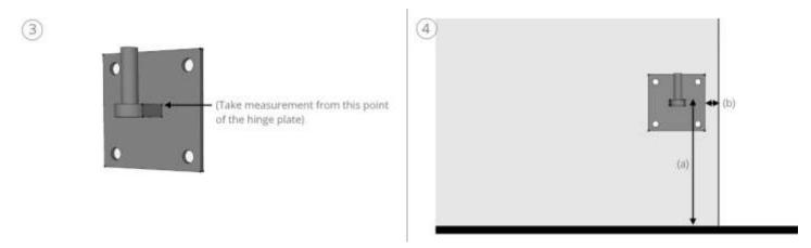
As we don't know what material customers are fixing the hinge plates to, we do not supply fixings for them. If into a solid pillar or wall, we would recommend Dewalt Hex Head Blue-Tip Screwbolts – 6 x 100mm. Please note: It is crucial to use the correct fixings due to weight of gate. If unsure, seek professional advice.
