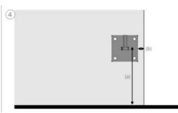
As we don't know what material customers are fixing the hinge plates to, we do not supply fixings for them. If into a solid pillar or wall, we would recommend Dewalt Hex Head Blue-Tip Screwbolts – 6 x 100mm. Please note: It is crucial to use the correct fixings due to weight of gate. If unsure, seek professional advice.
