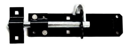
Select the position (usually best suited on top of the gate). Centralise on the horizontal brace (as looks better), mark holes, remove, drill pilot holes then fix. For added security, add a padlock.
