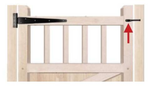
With the gate in the closed position, place the latch under the bar to check for position, mark holes, remove, drill pilot holes then attach with screws to post. Check the gate opens and closes securely. If needed adjust.
