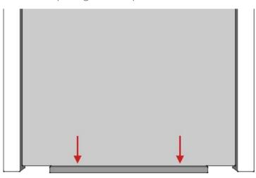
Ensure the gap between the mounting post and edge of gate is 10mm and mark the position of the top and bottom hinge on mounting post.
