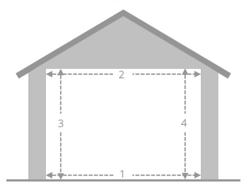
1: Use a tape measure to measure the **Garage Door's** opening from side to side near the floor of the garage. Measuring large dimensions of a **Garage Door** can be very tricky for one person. Ask a friend to help you hold one end of the measuring tape. Record this first measurement and all subsequent measurements on a piece of paper.
