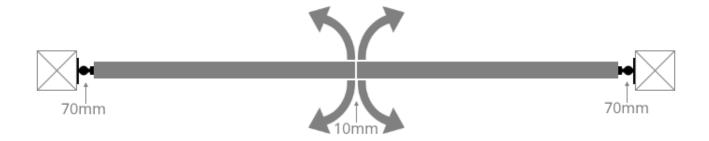
Gates can open both ways. Hinge plates mounted to inner face of post/ pillar. Gate to be mounted central between the posts.
