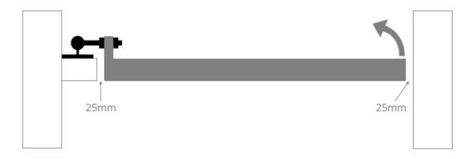
Alternative option if placing gate within two walls would be to mount a post to the wall. This set up would reduce the visible gap down the hinge side.
