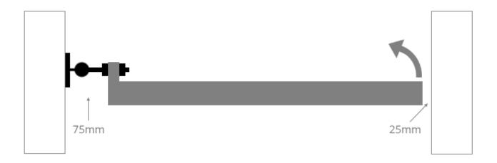
This set up example would be used if placing the gate in an alley way or similar. The allowance on the hinge side is greater and does create a visible see through section.
