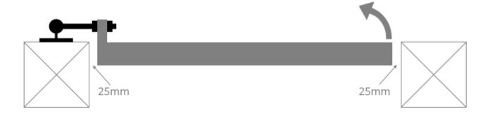
Gates to opens inwards towards property. Hinges mounted on rear of post/ pillar. Back edge of gate will be flush with the rear face of post/ pillar.
