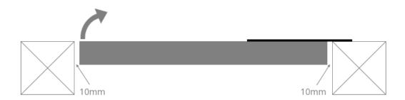
Gates to opens inwards towards property. Hinges mounted on rear of post/ pillar with the back edge of gate being inline with back of post/ pillar.
